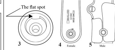
Fig. 3, (female) socket flat spot close-up
