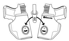
Moving the clip to the opposite side of the holster allows the user to adapt the holster for ambidextrous use.
