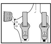
When worn in the appendix position (AIWB), the stabilizing claw/wing helps to push the butt of the gun closer to the body. The claw comes factory installed above the twin adjustable tension units.
