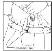
To use the Ultimate Stealth Clip start with your shirt tail outside your pants. Put the holster inside your pants with the bottom hook on the outside of your pants and behind your belt. Your belt will cover the arm of the bottom hook, leaving the top hook over the top of the belt.
