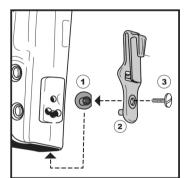
Insert the threaded brass post ① inside the holster while being careful to align the straight edge of the threaded post with the straight edge of the recessed dimple. Use your finger to hold the threaded brass post in place while installing the tuckable clip.
