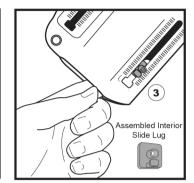
Insert the threaded post ① into the back of the Interior Slide Lug ② while being careful to align the straight edge of the threaded post with the straight edge of the recessed dimple.
