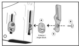
Snap the Exterior Angle Block 4 onto the threaded post of the Interior Slide Lug. Align the square dimple on back of the Exterior Angle Block with the square tab on the Interior Slide Lug.
