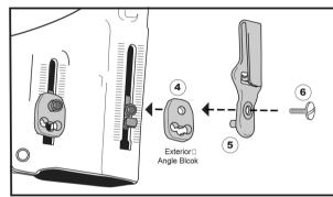
Snap the Exterior Angle Block 4 onto the threaded post of the Interior Slide Lug. Align the square dimple on back of the Exterior Angle Block with the square tab on the Interior Slide Lug.
