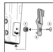
Insert the threaded brass post ① inside the holster while being careful to align the straight edge of the threaded post with the straight edge of the recessed dimple. Use your finger to hold the threaded brass post in place while installing the tuckable clip.
