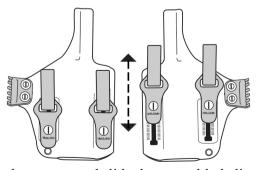
Loosen the screws and slide the assembled clip along the slots to change the ride height of the holster.
