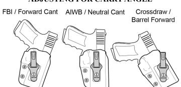
Changing the position of the stabilizing post on the back of the tuckable clip enables the user to fully adjust the cant/angle and carry position/ location.
