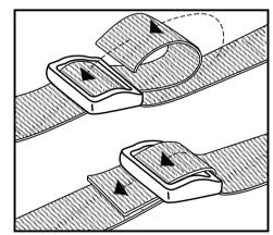
Tri-glide buckles may be locked into place (preventing shifting, sliding, etc.) by threading the tail-end of the strap back through the far end of the buckle, as shown. Straps with extra length after adjustment may be carefully trimmed and the edges melted to prevent fraying.
